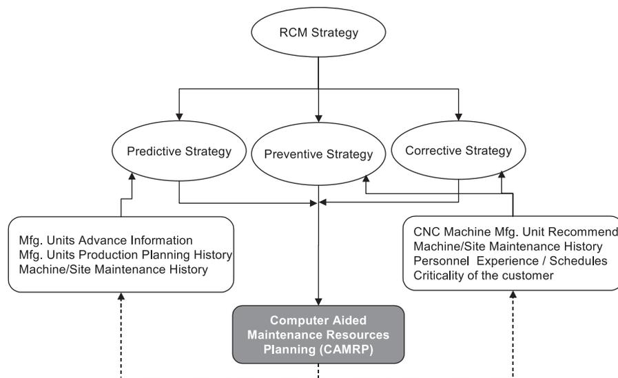
Fig. 2. Computer-aided maintenance resources planning supporting blocks.
