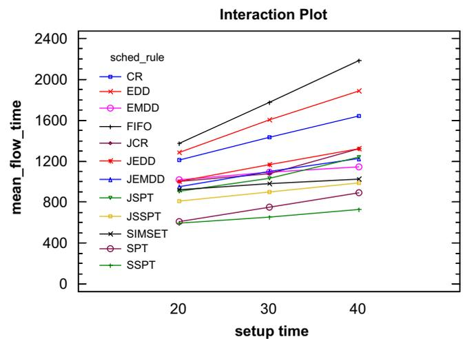
Fig. 6. Interaction plot for scenario 2—mean flow time.
