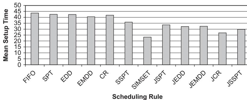
Fig. 4. Mean setup time ( $k = 5, s = 30\%$ ).
