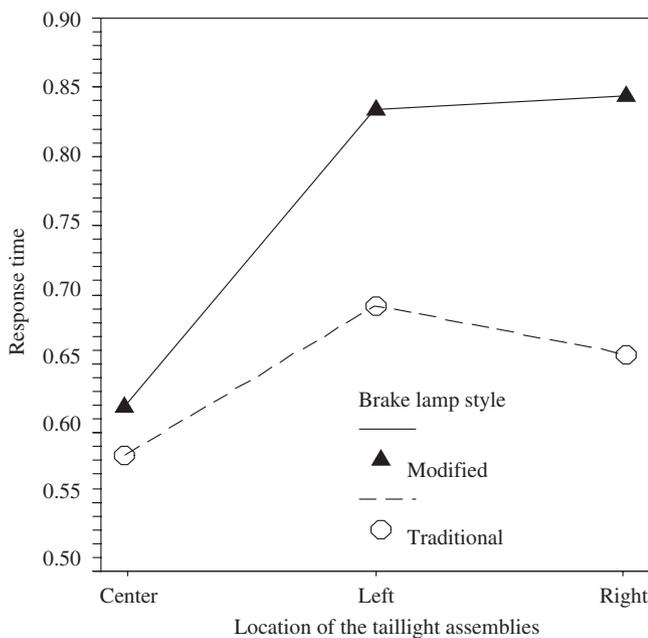
Fig. 5. Reaction times (s) to turn signals for two different types of brake lamps at three different locations.
