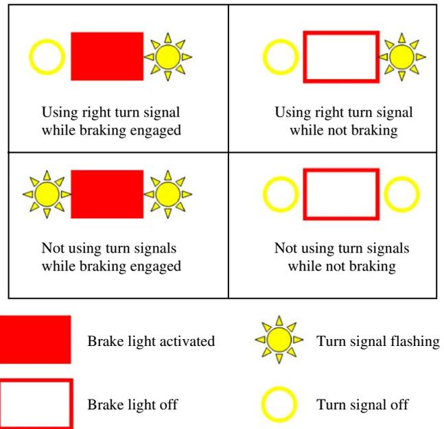
Fig. 1. The proposed functionalities for the supplemental brake lamp of motorcycles. Note that only the right turn signal on or off scenarios are depicted in this figure. The left turn signal on or off scenarios have the same effect.
