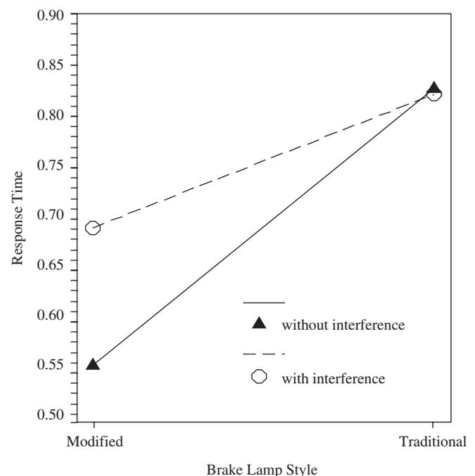
Fig. 3. Reaction times (s) to brake signals for two different types of brake lamps, with or without using the normal function of turn signals.
