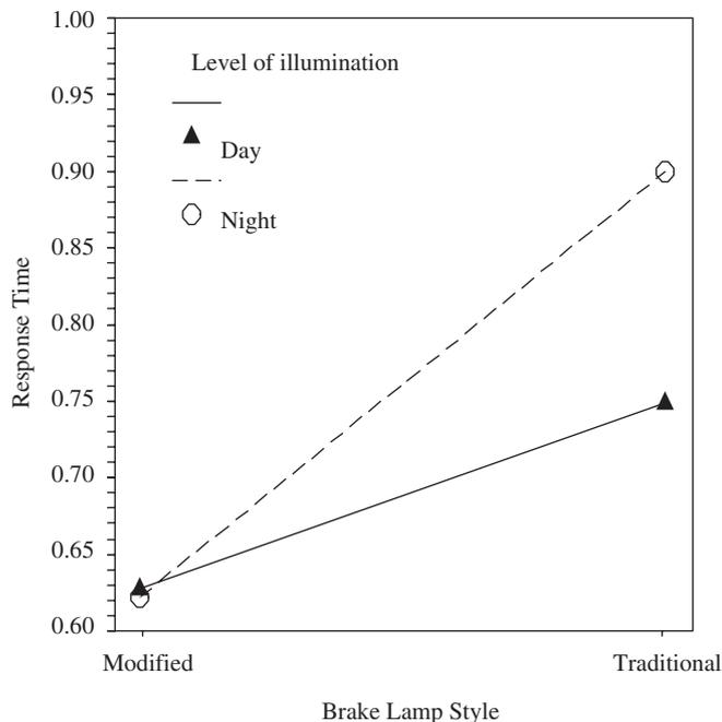
Fig. 4. Reaction times (s) to brake signals for two different types of brake lamps at different levels of illumination.
